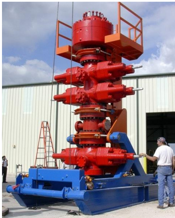
Figura 4: Blowout Preventer (BOP).
